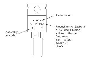
Example: This is a xxxxx with assembly lot code AC, assembled on WW 19, 2001 in the assembly line "X"
